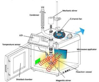
**Fig. 1**: The microwave assisted transesterification setup by Lin et al., (2014)
